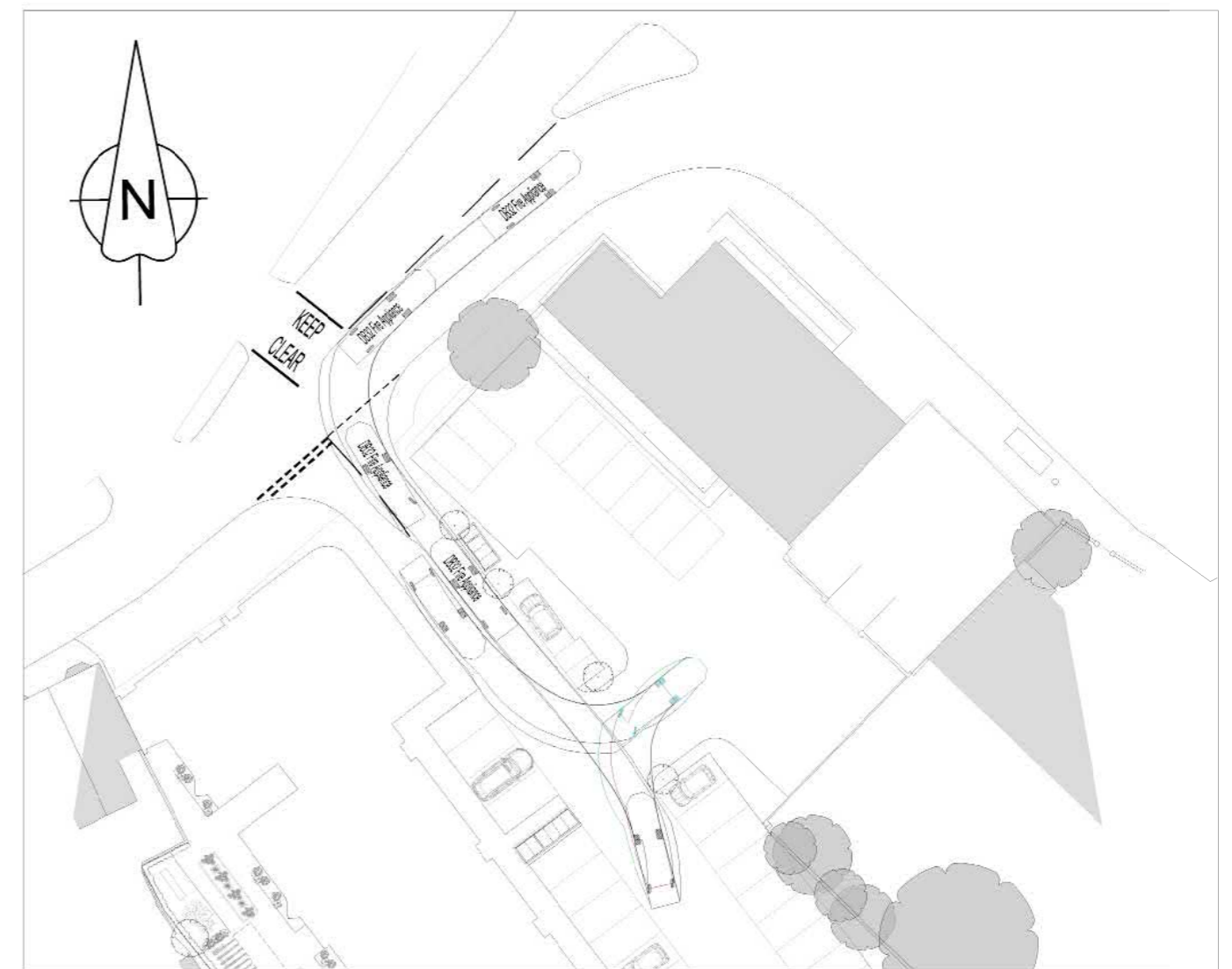
FIRE TENDER TURNING LEFT INTO SITE & TURNING TO EXIT 1:500@A2
