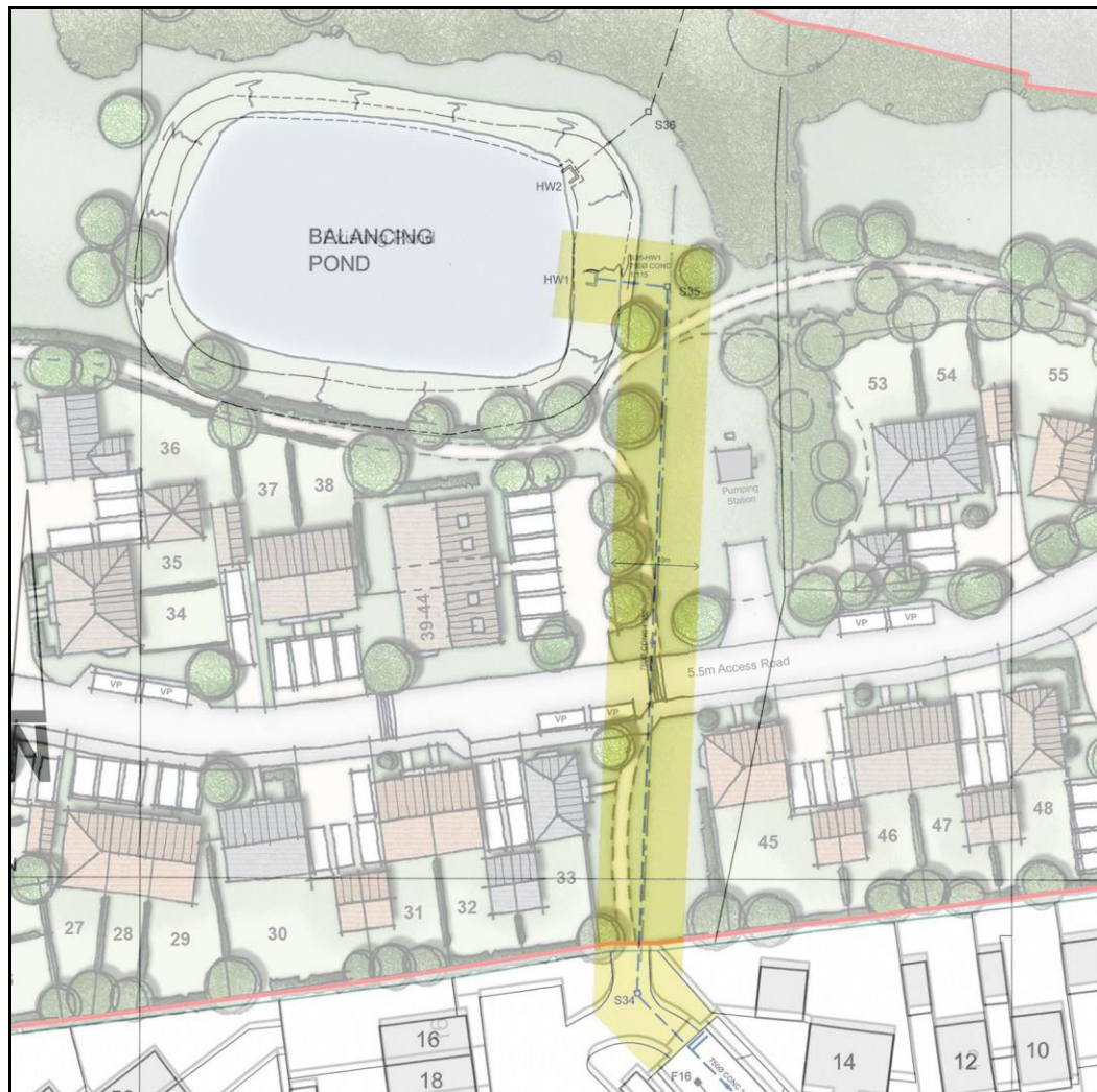
Figure 10. Existing surface water connection to the on-site attenuation pond overlaid on the illustrative development layout.
