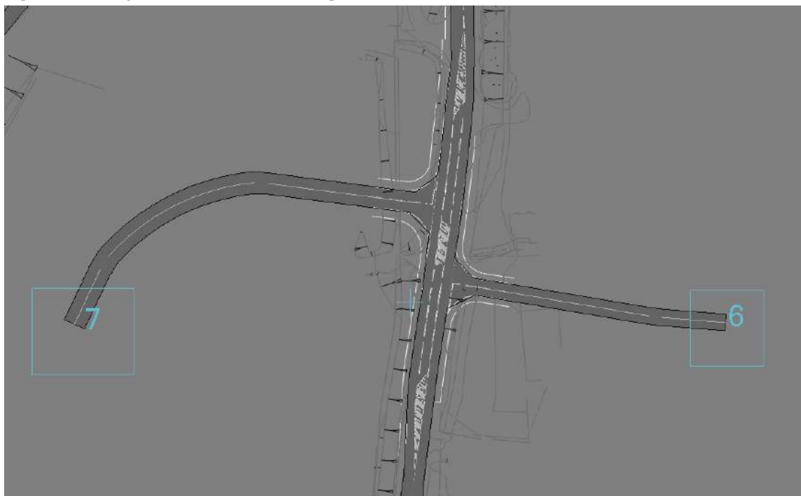
Figure 5.2: Proposed North West Sittingbourne Site Access Junction Paramics Plot
