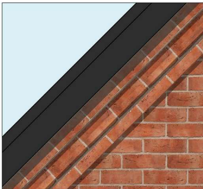
clipped eaves & dentil course
