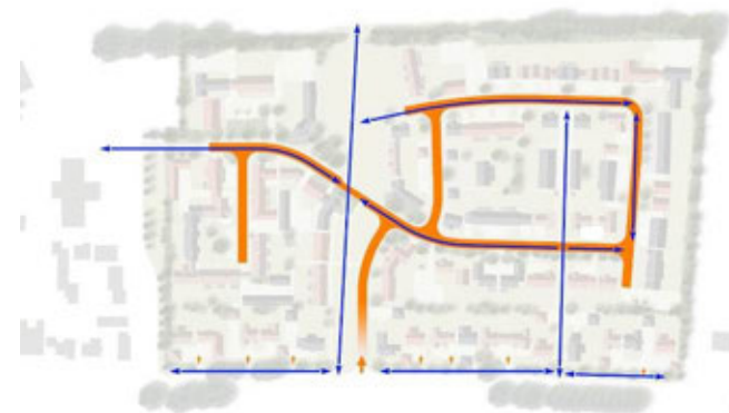
Fig.9 Site Access - Pedestrian routes in blue and vehicle access routes in orange
