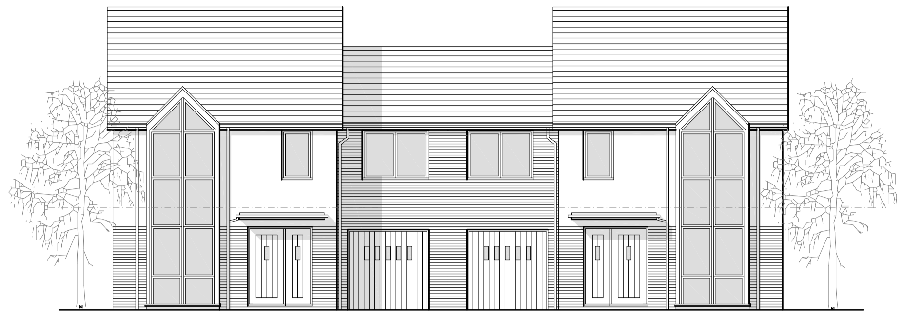
Front Elevation - Pair attached by garage side.
