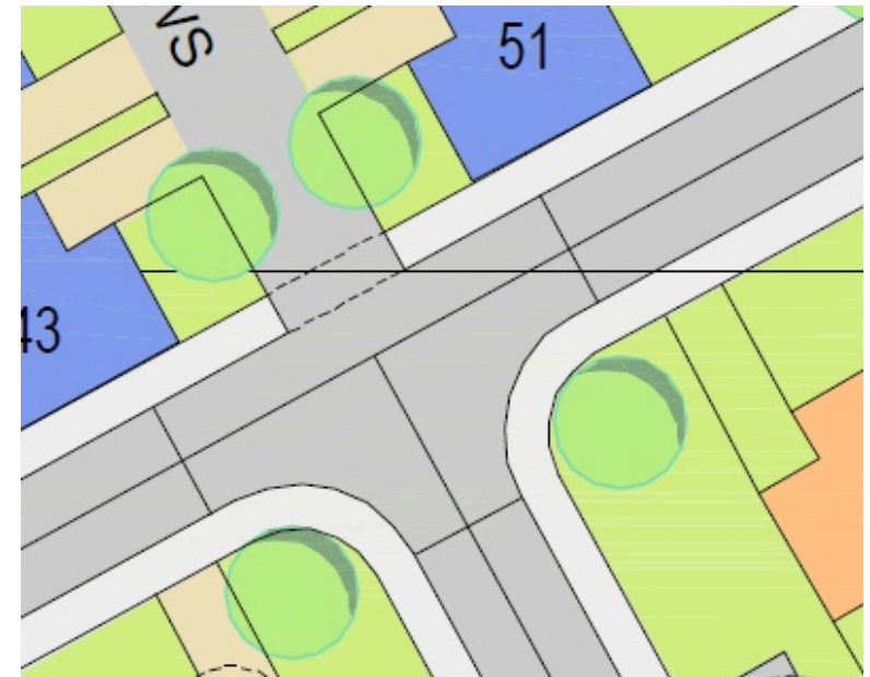
A typical junction with 4m radius kerb lines & raised table.
