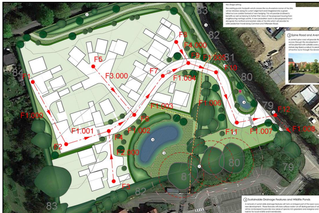
Figure 6. Illustrative foul drainage layout.
