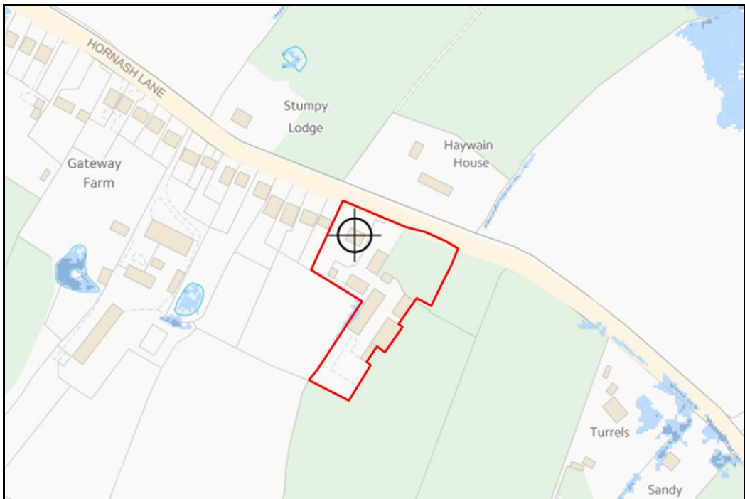
Figure 13. Surface water flood depth map for the high risk flood event with the site edged red.
