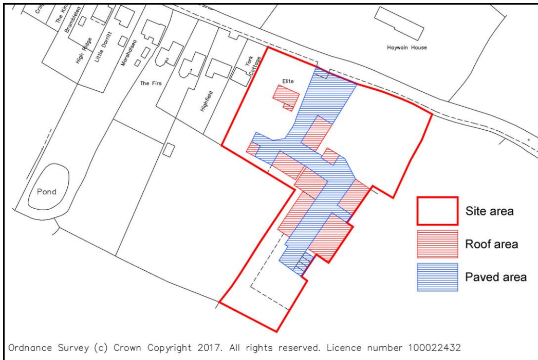
Figure 8. Existing impermeable areas.
