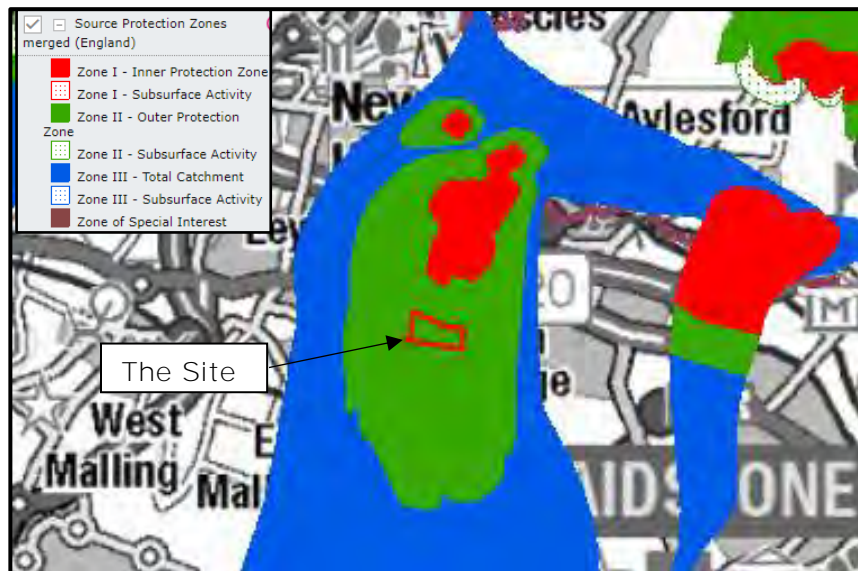
Figure 2.4 Groundwater Source Protection Zone
