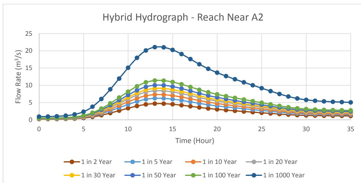
**Figure 1-4 Hybrid Flood Hydrograph – Reach Near M2**
