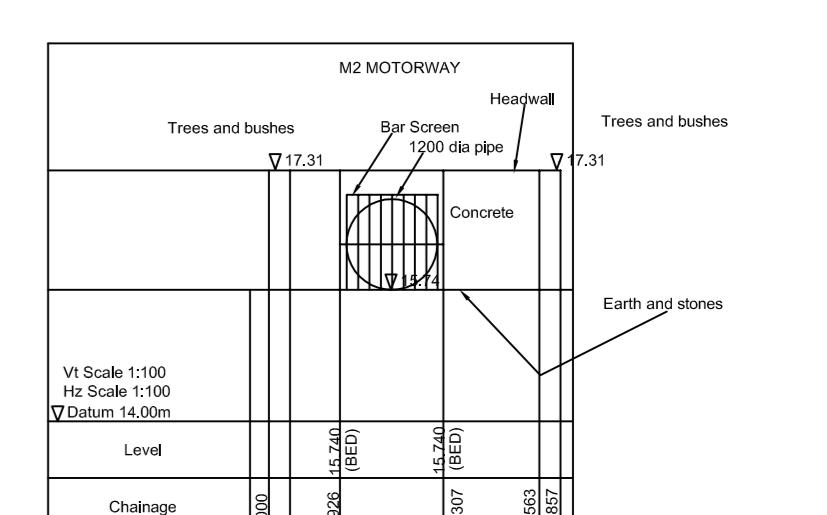
1. This site level survey has been undertaken to the Ordnance Survey National Grid (OSGB36) via GNSS/GLO/NASS RTK.
