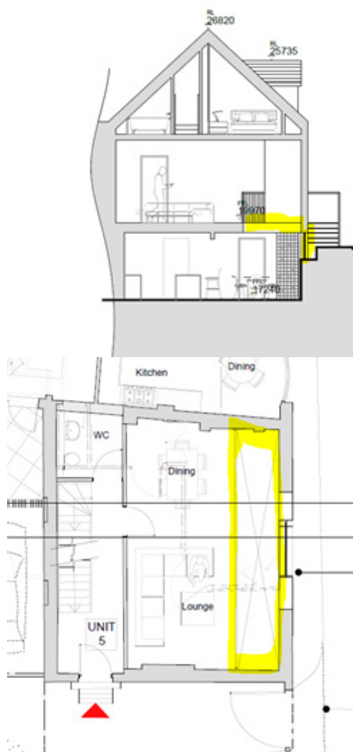
Figure 9: Cross section of unit 7 and ground floor plan of unit 5 (yellow highlight area shows lightwell)
