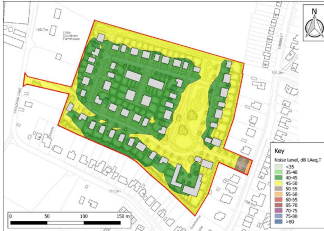
Figure B3: Night-time Noise Contour, 1.5m
