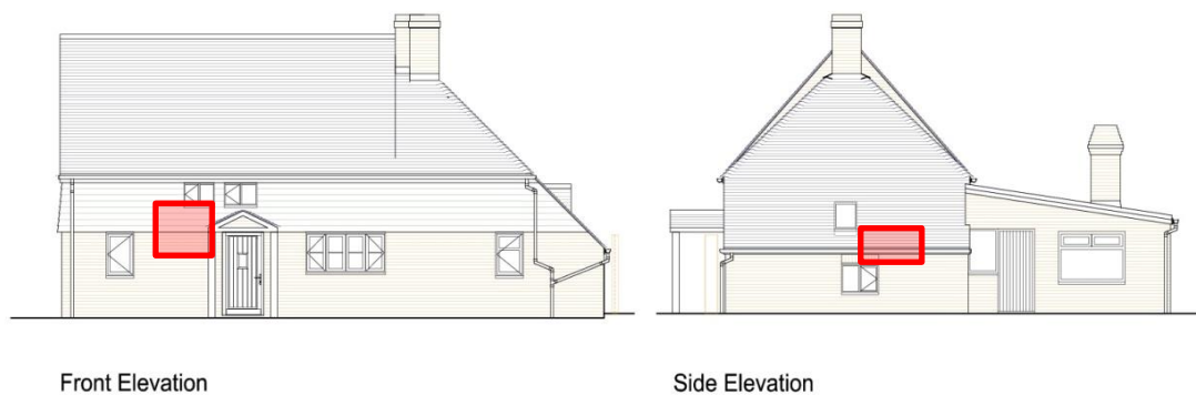
Figure 1: Suggested locations for pilot holes to investigate the material used for the infill panels
