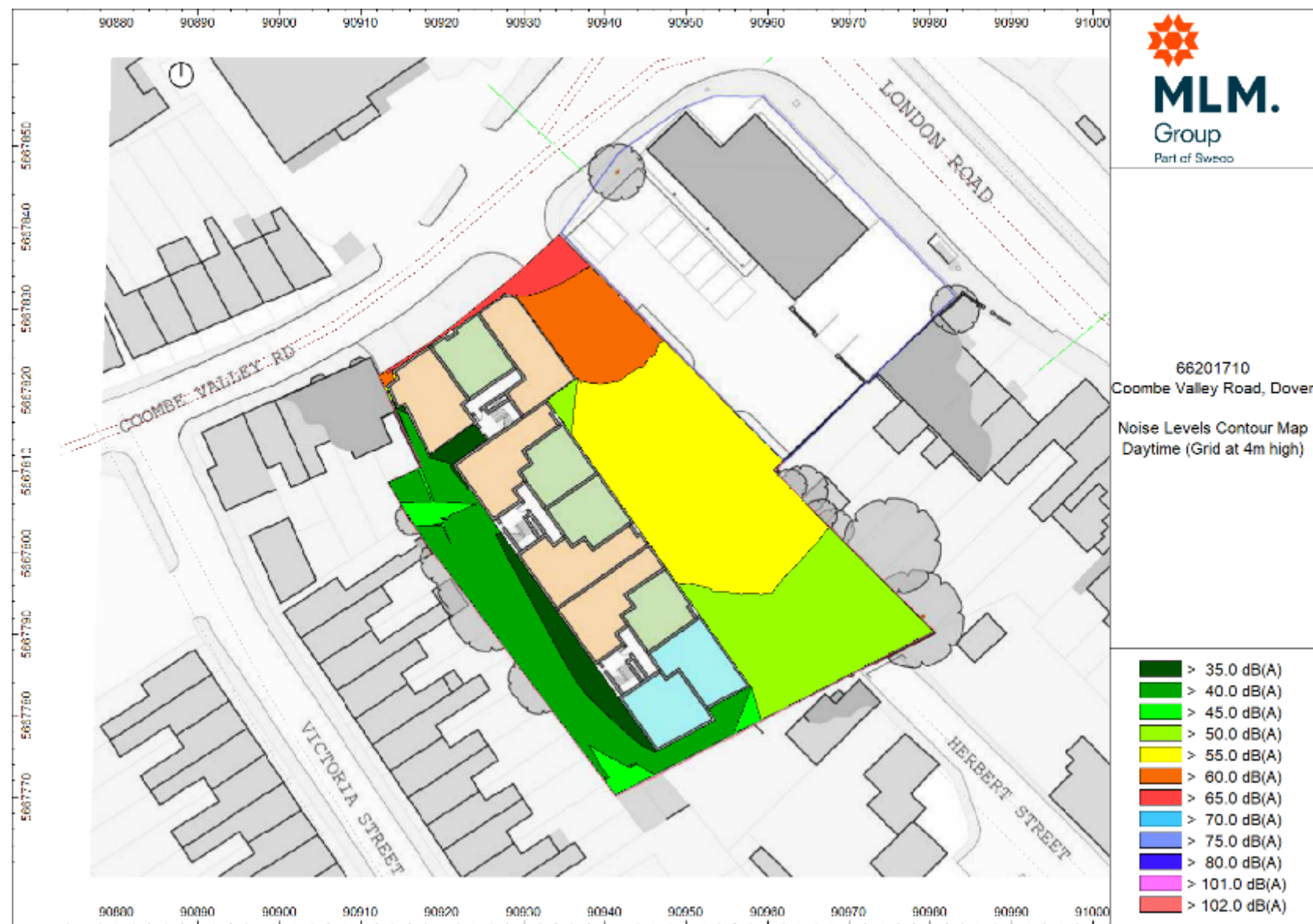
Figure D.3: Noise Contour Map with Concept Masterplan – L_{Aeq,T} Daytime (Grid at 4m high)
