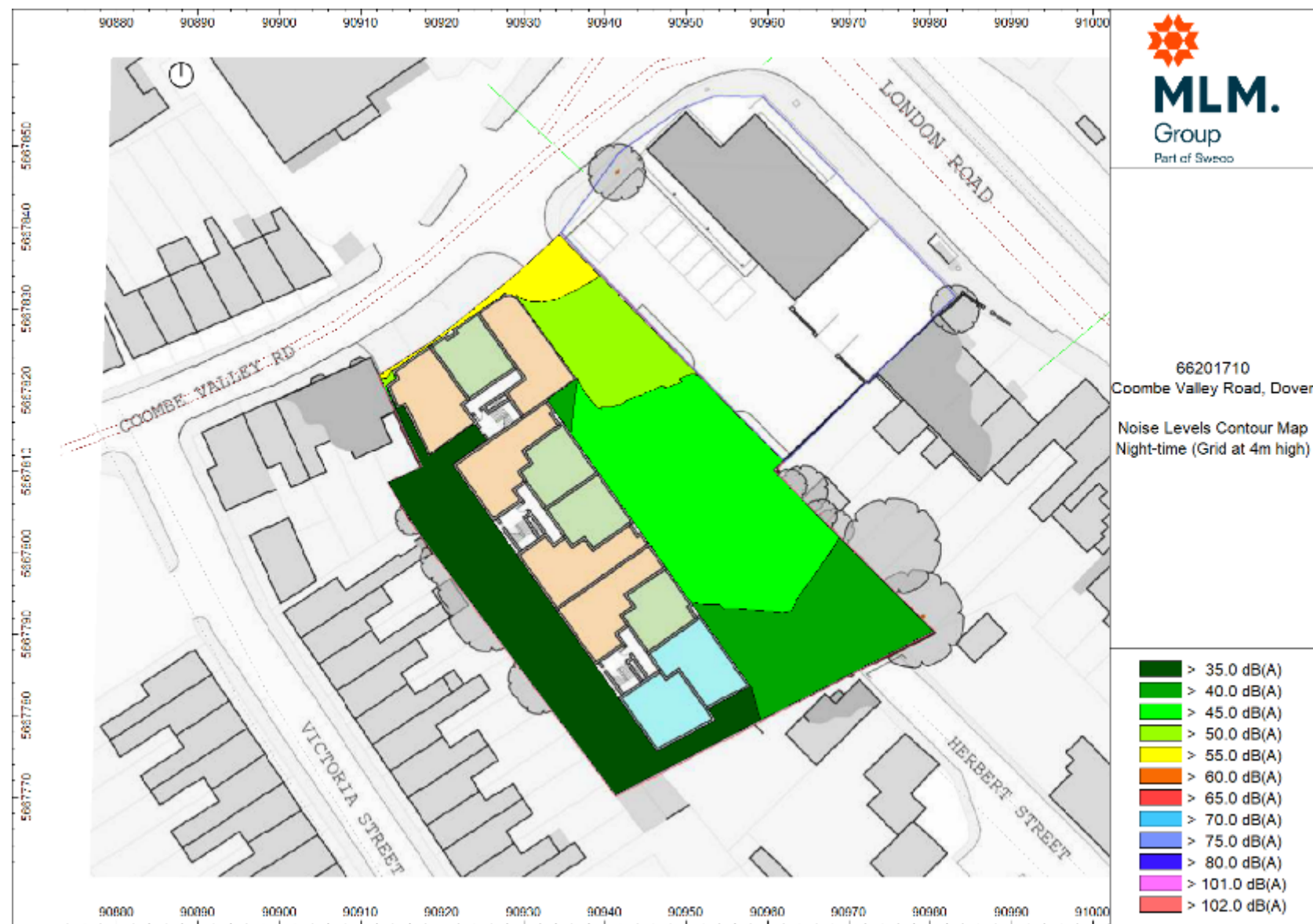
Figure D.4: Noise Contour Map with Concept Masterplan – L_{Aeq,T} Night-time (Grid at 4m high)
