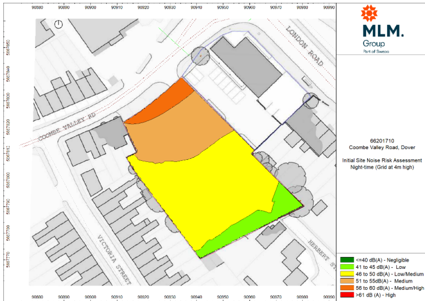
Figure D.2: Initial Site Noise Risk Assessment – L_{Aeq,T} Night-time (Grid at 4m high)
