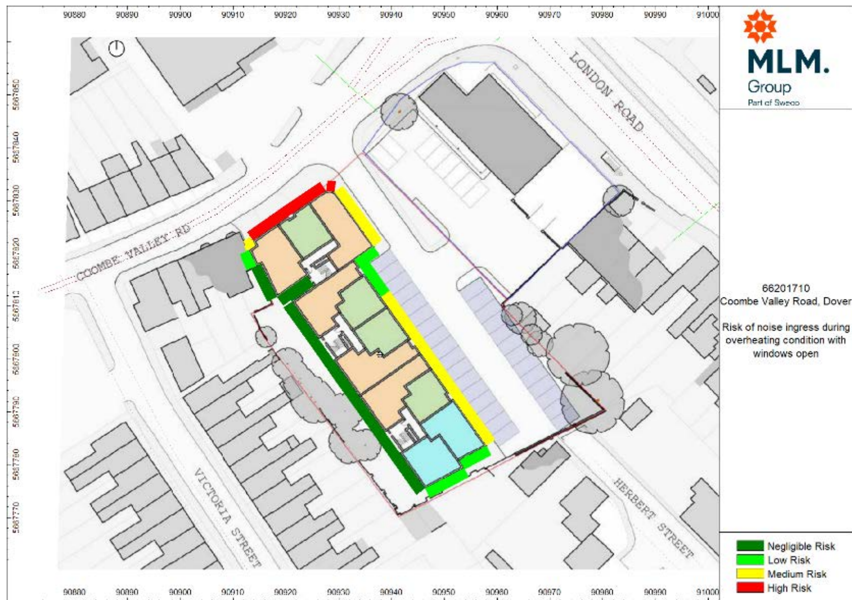
Figure D.8: Risk of Noise Ingress during Overheating Condition
