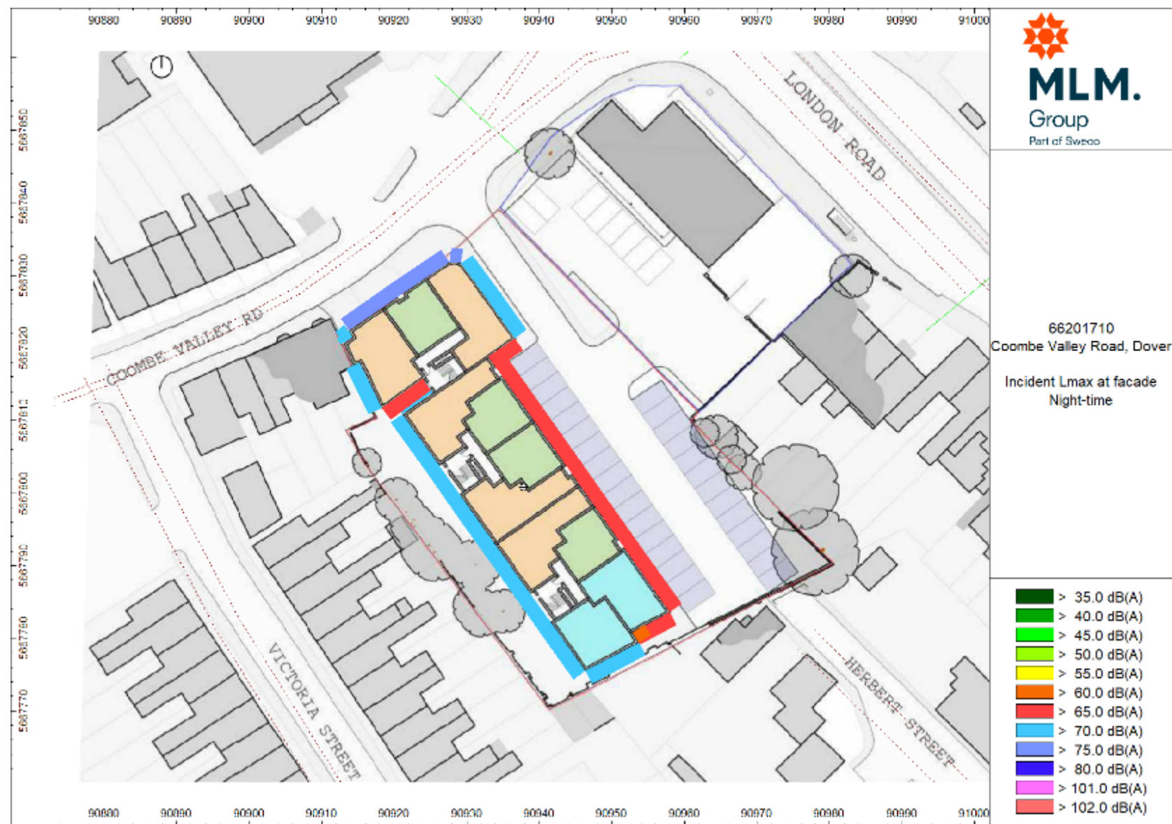
Figure D.5: Façade Incident Maximum Noise Levels – L_{Amax} Night-time (Grid at 4m high)
