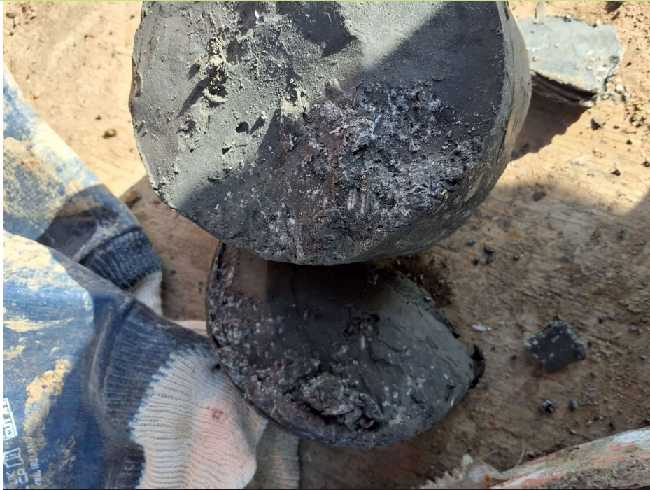
Plate 5: BH203 unweathered London Clay
