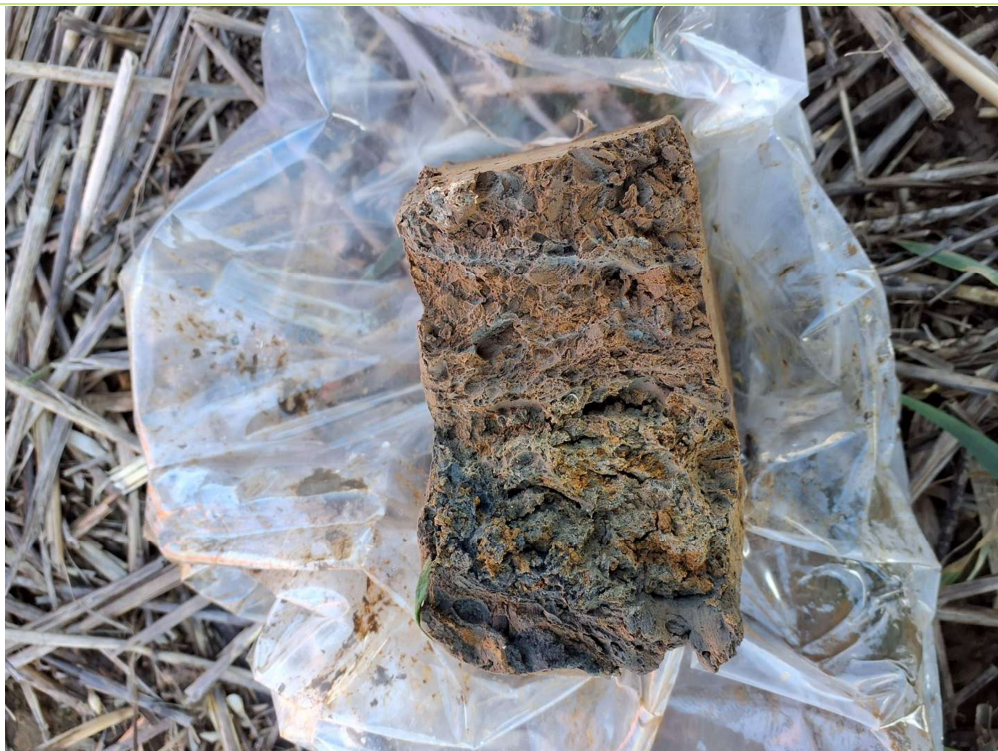
Plate 4: BH203 weathered London Clay
