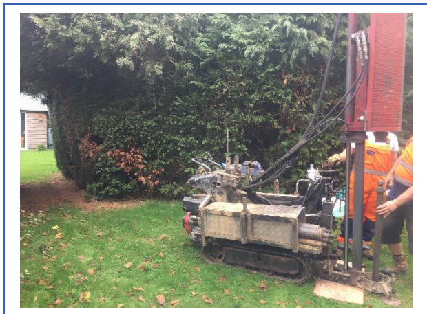
Windowless sampling rig used on site
