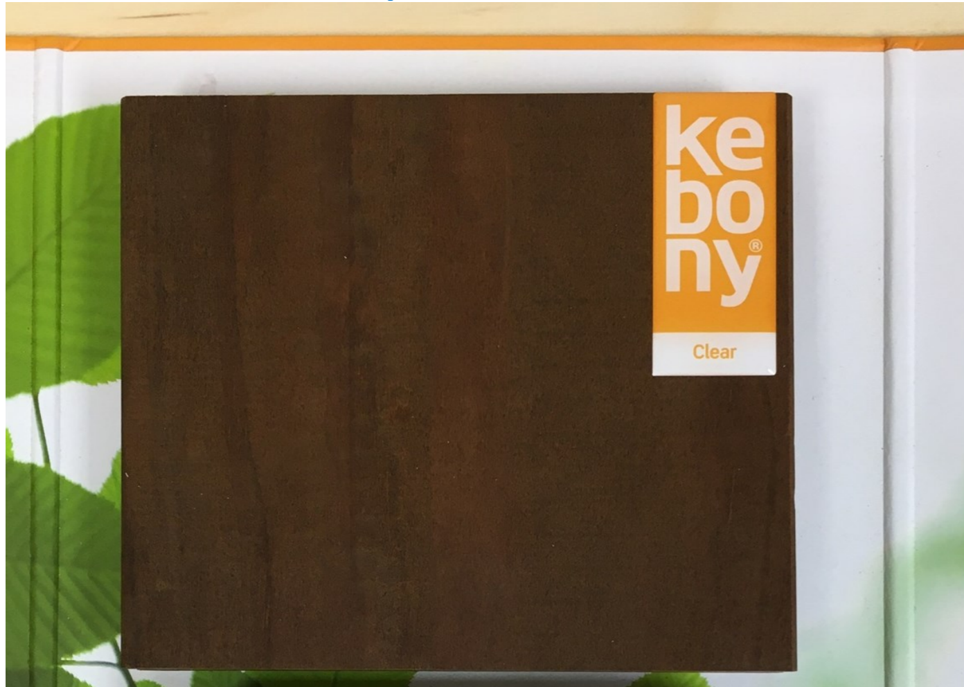
Fig. 20 Sample of proposed timber cladding (new, prior to natural weathering)
