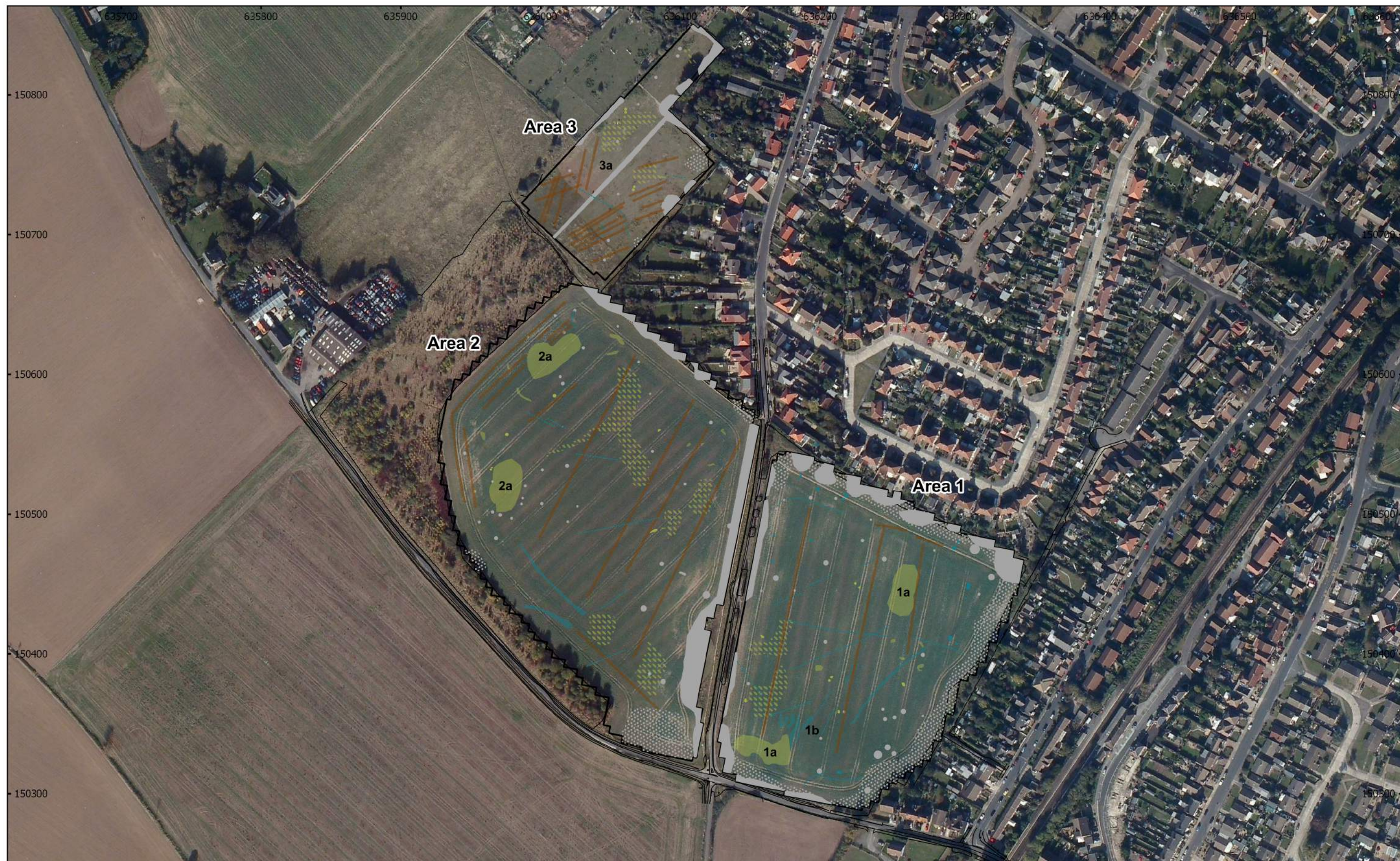
MSTR121 - Land at Cross Road, Deal, Kent Figure 5 - Magnetic Interpretation over Satellite Imagery 1:2500 @ A3 Copyright Magnitude Surveys Ltd 2017 Contains satellite Imagery: © 2017 Bing
