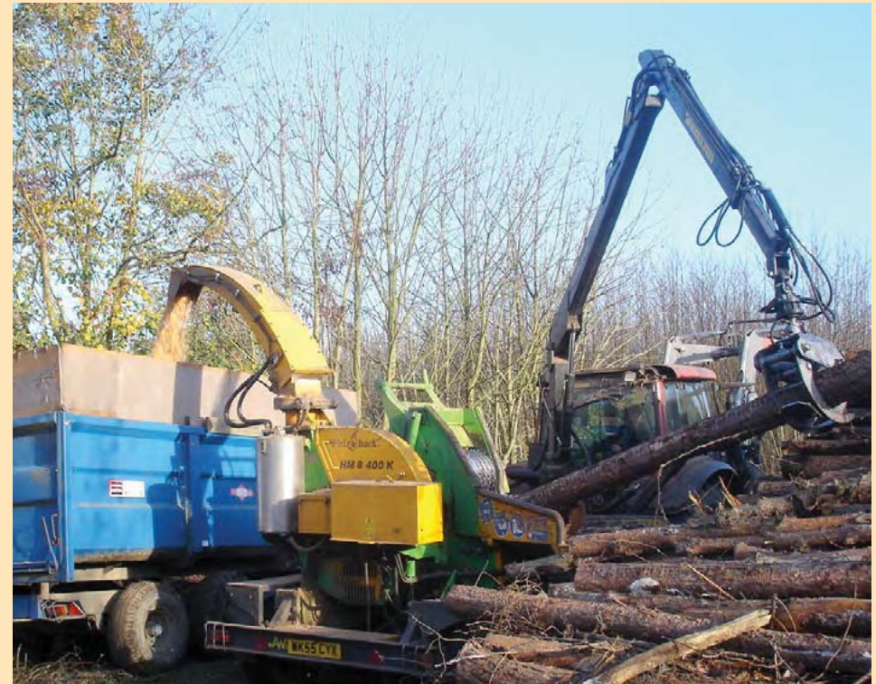
Wood chipping in action. The woodland resource provides an excellent opportunity for biomass energy in the form of wood chip.
